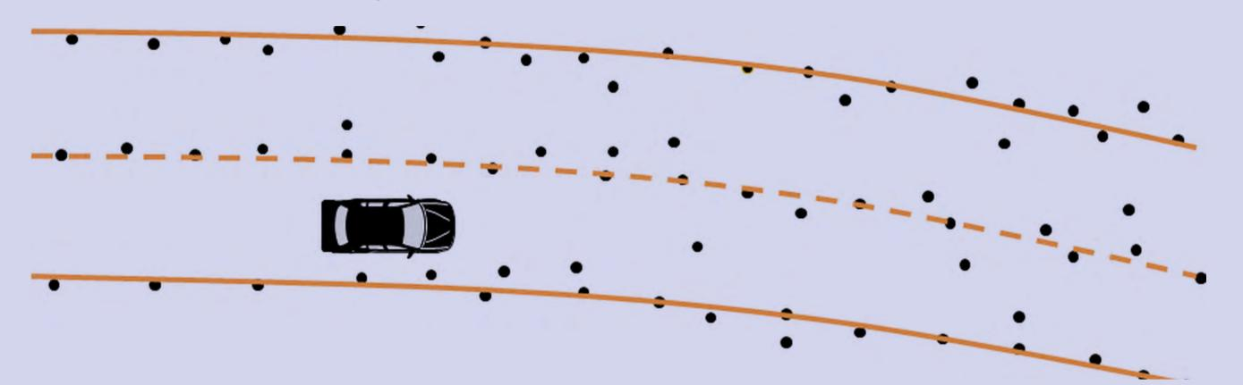
The resulting sensor-based road model is transformed into a generic model free representation for further steps
