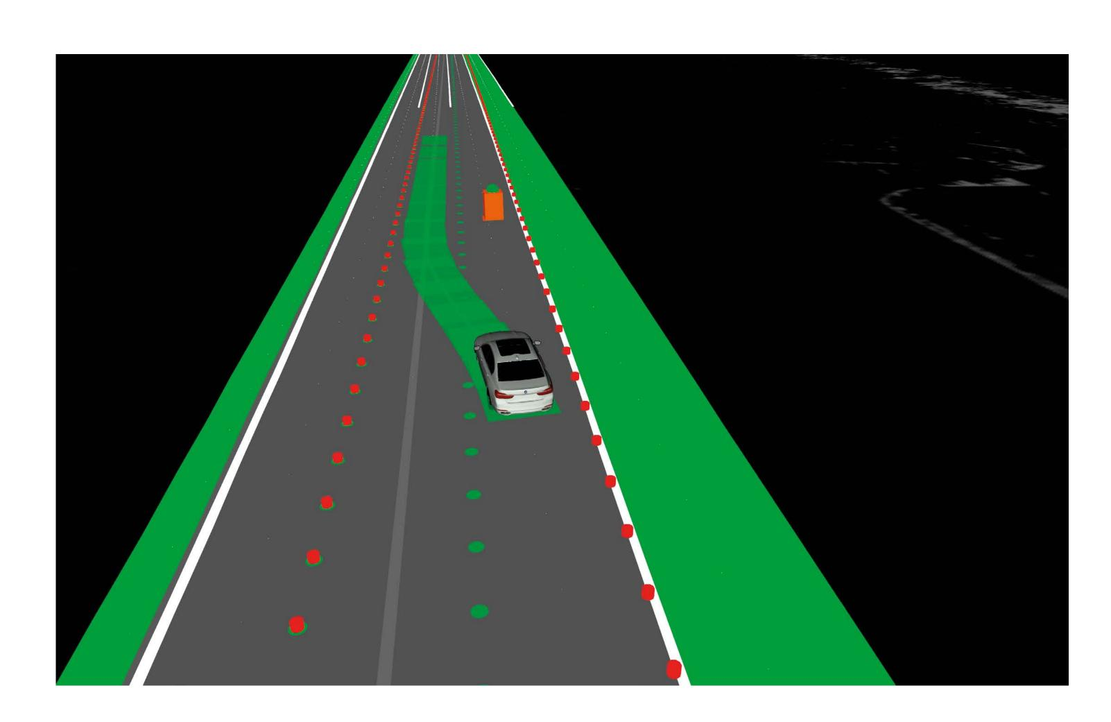
4. After passing the obstacle, the vehicle will change back to the rightmost lane, observing the obligation to drive on the righthand side.
